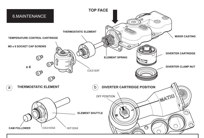
IMPORTANT. Before commencing maintenance on the mixer turn off the hot and cold inlet supplies. When maintenance is complete ensure that the mixer is checked and fully commissioned before use.
