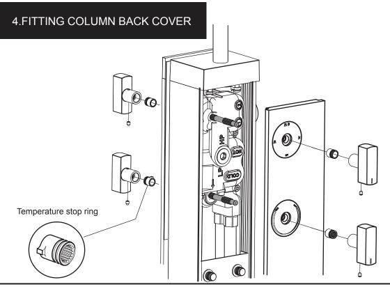
Remove the Handles. Fit the Shower column back cover as shown in the installation instructions. Check that the spindles protrude equally from the inside and outside face of the column and align through the holes. The spindles can be removed by pushing them through the column and pulling them from the inside.
