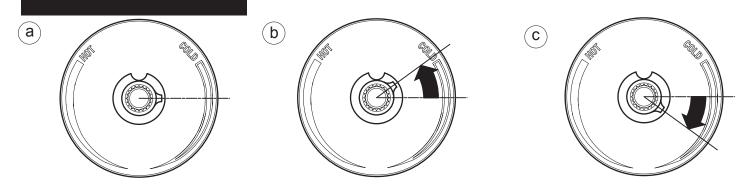
Important: The maximum hot water temperature must be checked and reset if necessary, prior to the mixer being commissioned to avoid scalding. Check that the hot water system is operational and that the hot water supply has reached the optimum temperature.
